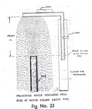
MEASURING WATER DISCHARGE FROM RISE OF WATER COLUMN ABOVE PIPE
