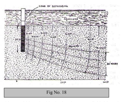
The problem could be solved by having the screen divided into shorter lengths and alternated with blank pipes. Figures 19 and 20 below give the pattern of reducing the convergence of flow.
