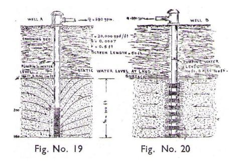
Hither to the department has worked out total length of sweet water column and developed only 60 % of it. Care has been taken to put a long filter, but theoretically it appears that breaking of filter and alternating it with blank pipes is better. Such a tube well can increase specific capacity by even 50%
